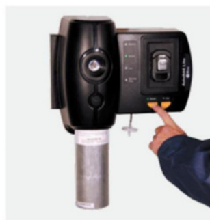
Bump testing ToxiRAE 3 with AutoRAE Lite Bump Test and Calibration Station
